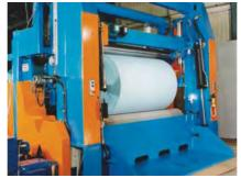
General purpose two drum winder incorporating individual drum drives, automatic nip and tension control for processing all types of paper and board. The slitting is located at the rear of the machine with dual spreader rolls for slit strip separation.
