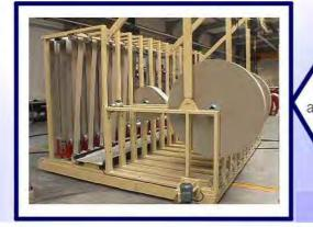
The ATC-90 unwinder includes a dancing roll festoon for a manual flying splicing of the plies at full speed. It is specially designed for heavy and stiff board and has larger diameter idlers, a 90° paper twisting system (twice 45°) and a walkway to collect the empty shafts.
