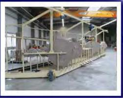
The **unwinder** is the most standard unwinding system. It is compact, has a 45° paper twisting system and a walkway to collect the empty shafts.
